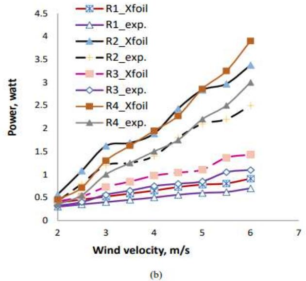
Figure 7. (a) Torque distribution of the R1, R2, R3, and R4 rotors with new air foil blade section. (b) Power distributions of the R1, R2, R3, and R4 rotors at different wind speed.
