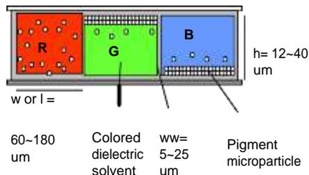
**Figure 1** Schematic cross-section of a color Microcup® EPD. Each microcup is isolated and seamlessly top-sealed.
