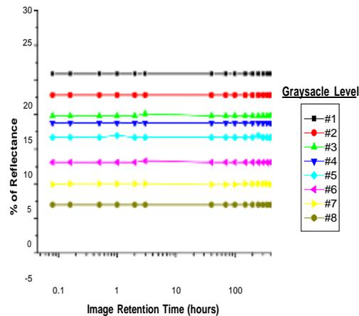
Figure 5 Grayscale stability of a typical Microcup® PMEPD at the power-off state.
