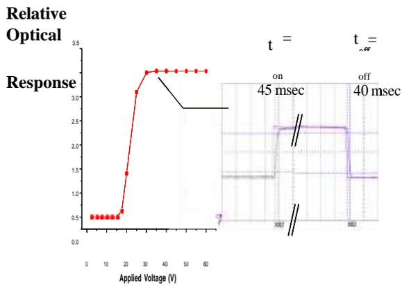
Figure 4 Electro-optical response of a typical Microcup® PMEPD.
