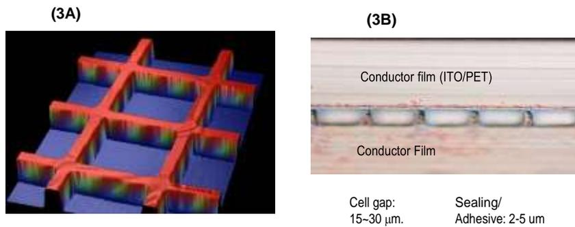
**Figure 3** A typical Microcup® structure (3A) and the cross-section of filled and sealed sample (3B).
