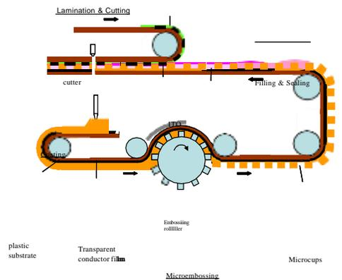
**Figure 2** Schematic process flow of the SiPix roll-to-roll electronic paper manufacturing process
