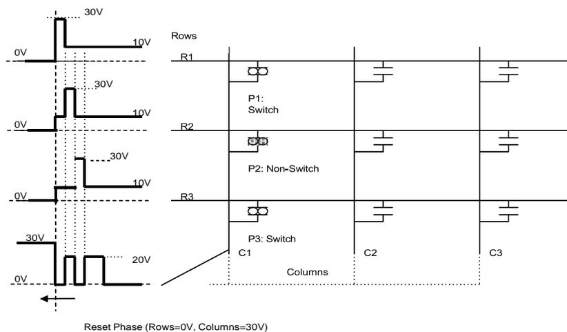
**Figure 6** Driving waveforms of a Passive Matrix Microcup® EPD
