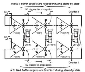
Fig. 5. Block diagram of the proposed fine TDC
