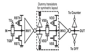
Fig. 6. Detailed schematic of the PSB.
