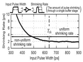
Fig. 3. Simulated PS rate versus input pulse width.
