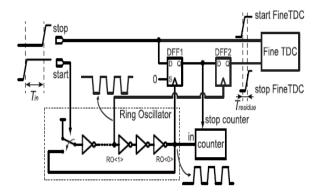
Fig. 9. Block diagram of the proposed TS TDC.
