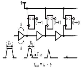
Fig. 2. Simplified schematic of a typical PS TDC.
