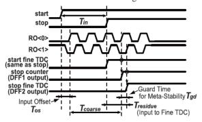
Fig. 10. Timing diagram of the proposed TS TDC.
