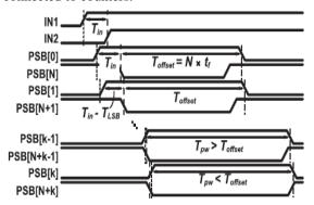
Fig. 7. Timing diagram of the PS TDC.
