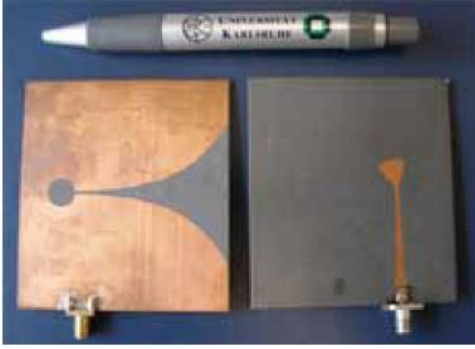
Fig. 6. Aperture coupled Vivaldi antenna. (Left) Top view ;( right) bottom view with feed line. Substrate size 75 _ 78 mm2.
