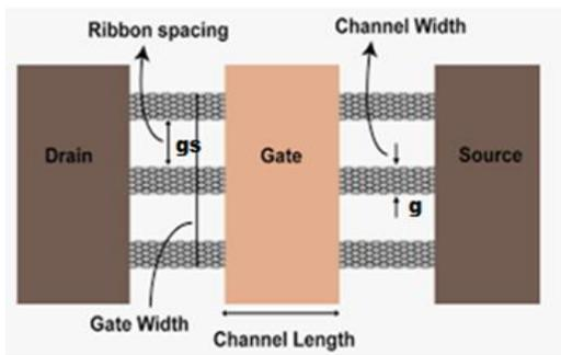
Figure 1b: Cross sectional view of a GNRFET
