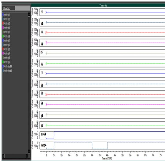
Figure 15.a Simulation results of row and column address selection of 64x64 SRAM
