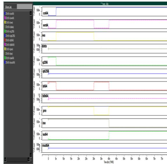
Figure 15.c: Logic 0 simulation results of 64x64 SRAM
