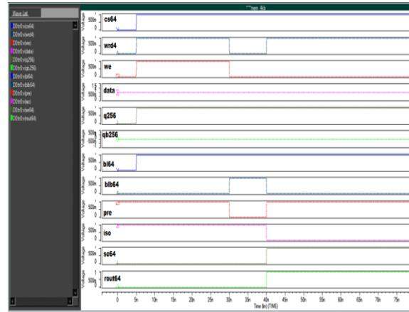
Figure 15.b: Logic 1 simulation results of 64x64 SRAM array
