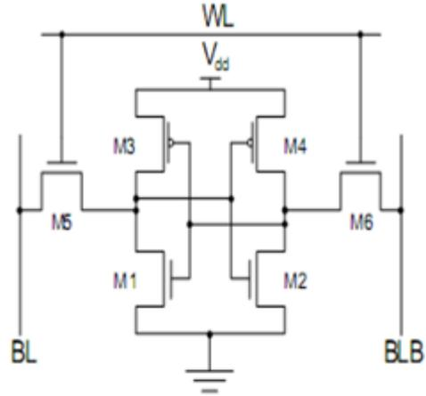
Figure 4: 6T SRAM cell in CMOS technology
