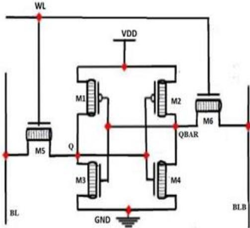
Figure 5: 6T SRAM cell in GNRFET technology
