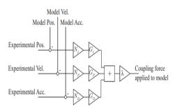
As shown in Fig. 4, the homotropy coupling term has been implemented in Maples.
