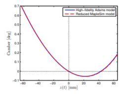
Verification of front camber, shown in Fig.2 An analytical method for determining how much each bushing in the SLEKQ model affects the overall system behaviour would be prohibitively time-consuming and inaccurate, making this a perfect chance to use a parameter identification technique. The damping force is specified by the following piecewise linear function:
