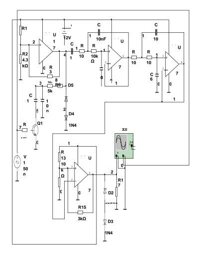
Fig. 7. Circuit for simulation study of the synthesized FSK modulator-demodulator.
