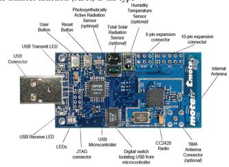
Fig. 2 Picture of Tmote node (top layer) [10]
