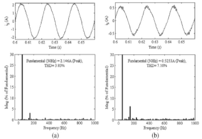
Fig. 7. Harmonic spectra of supply current at rated supply voltage and rated loading on BLDC motor for a dc link voltage of (a) 200 V and (b) 50 V.
