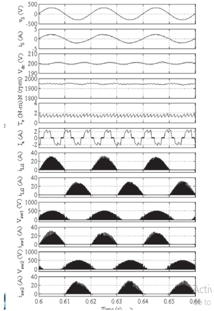
Fig. 6. Steady-state performance of the proposed BLDC motor drive at rated conditions.
