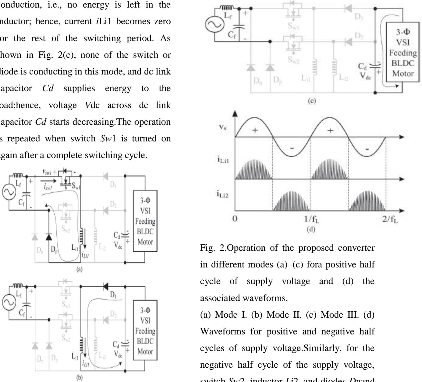
Fig. 2. Operation of the proposed converter in different modes (a)–(c) for a positive half cycle of supply voltage and (d) the associated waveforms.
