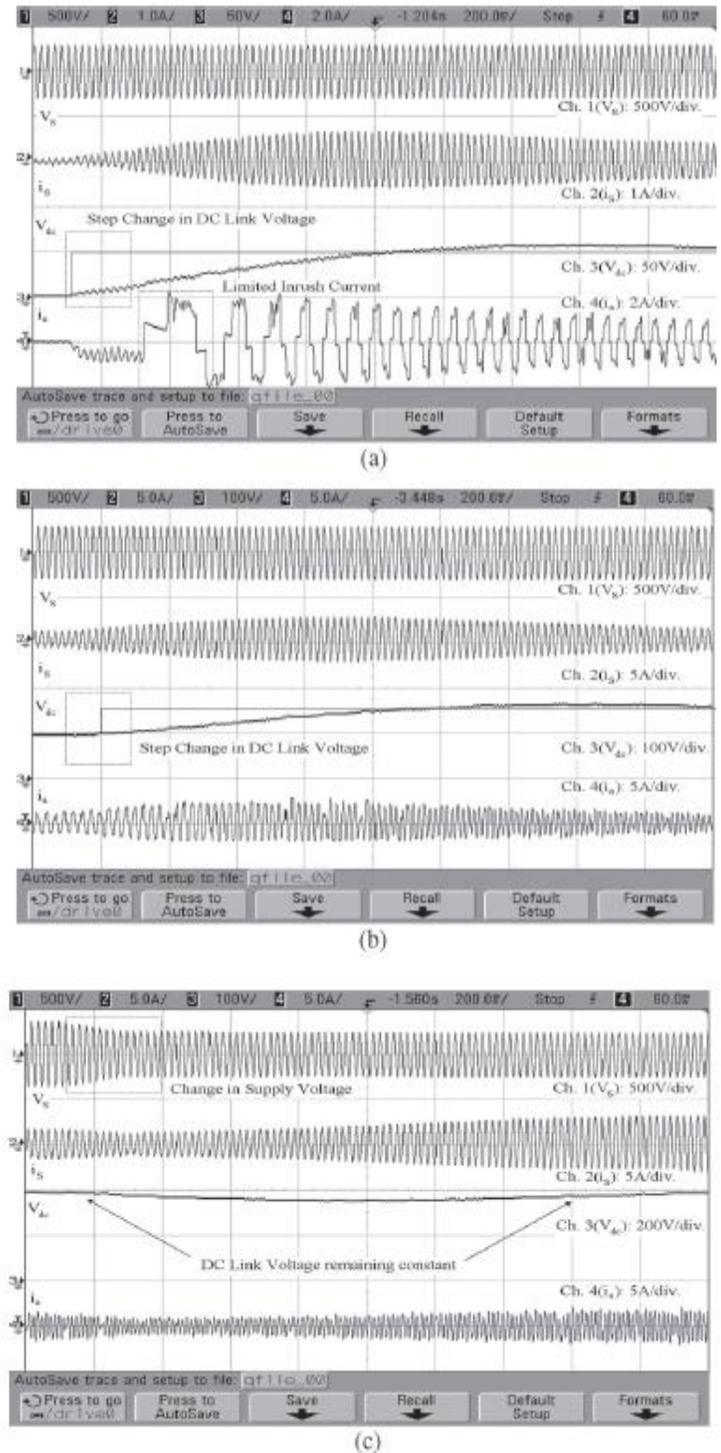
Fig. 13. Dynamic behavior of the proposed BLDC motor drive during (a) starting at dc link voltage of 50 V, (b) step change in dc link voltage from 100 to 150 V, and (c)
