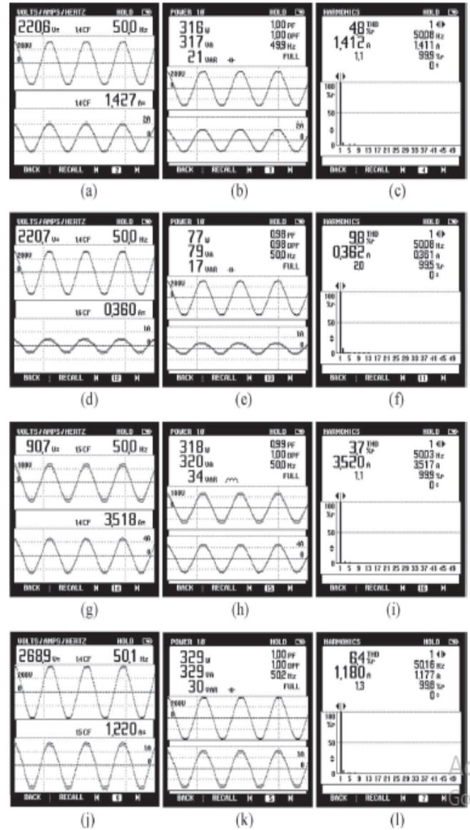
Fig. 14. Power quality indices and performance parameters ( $v_s$ ,  $i_s$ ,  $P_{ac}$ ,  $P_a$ ,  $P_r$ , PF, DPF, CF, and harmonic spectrum of  $i_s$ ) of proposed BLDC motor drive at rated load on BLDC motor with (a)–(c) dc link voltage as 200 V and supply voltage as 220 V, (d)–(f) dc link voltage as 50 V and supply voltage as 220 V, (g)–(i) dc link voltage as 200 V and supply voltage as 90 V, and (j)–
