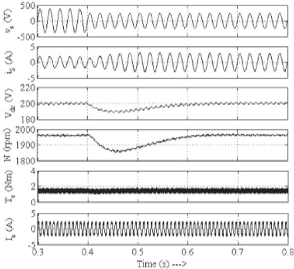
Fig. 8. Dynamic performance of proposed BLDC motor drive during (a) starting, (b) speed control, and (c) supply voltage variation at rated conditions.
