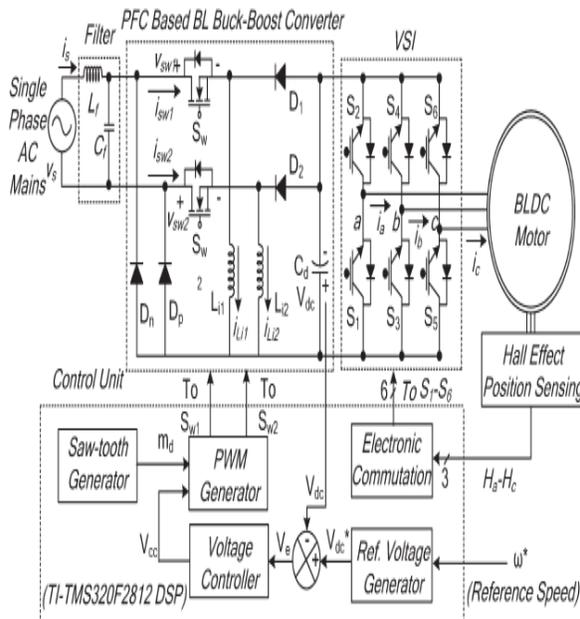
Fig. 1. Proposed BLDC motor drive with front-end BL buck–boost converter Gopalarathnam and Toliyat [12] but has higher losses in VSI due to PWM switching and a higher number of current and voltage sensors which restricts its applicability in low-cost application. Singh and Singh [8]
