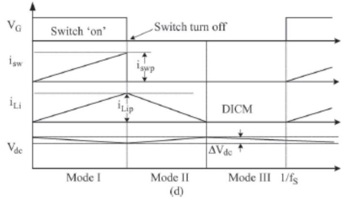
Fig. 3. Operation of the proposed converter in different modes (a)–(c) for a negative half cycle of supply voltage and (d) the associated waveforms.
