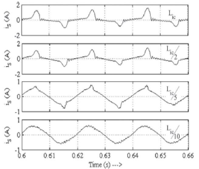
Fig. 4. Supply current at the rated load on BLDC motor for different values of input side inductors with supply voltage as 220 V and dc link voltage as 50 V.
