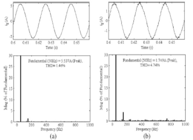
Fig. 9. Harmonic spectra of supply current at rated loading on BLDC motor with dc link voltage as 200 V and supply voltage as (a) 90 V and (b) 270 V.
