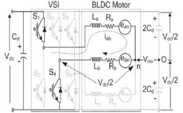
Fig. 5. Operation of a VSI-fed BLDC motor when switches  $S_1$  and  $S_4$  are conducting.
