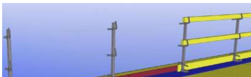
Fig. 4. BIM-based falling prevention planning: safety railings in edges of cast-in-place slabs (Kiviniemi et al., 2011).
