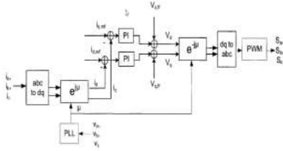
Fig. 4. PWM linear feedback current control scheme
