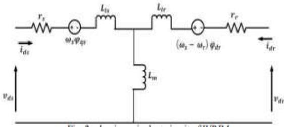
Fig. 2. d-axis equivalent circuit of WRIM
