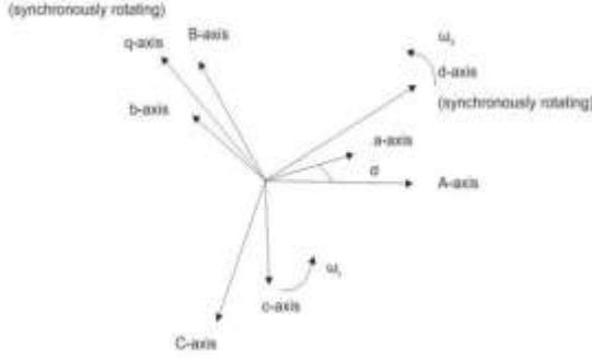
Fig. 1. Reference system used in DFIG
