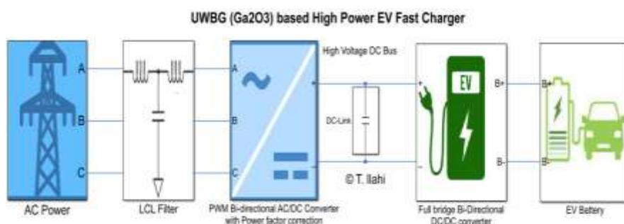
**FIGURE 2.** Simscape MATLAB model of UWBG high power EV fast charger
