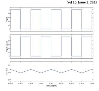
**FIGURE 11.** Switching signals for  $S_1$ ,  $S_2$ ,  $S_3$ ,  $S_4$  and inductor currents in boost mode of operation.
