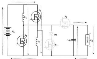
controlledswitches  $S_1$ ,  $S_2$ ,  $S_3$  and  $S_4$ . The switches  $S_1$ ,  $S_2$  and  $S_3$  are operated through the PWMcontrol. Typical waveforms of the proposed HG BDC in boost mode for continuous conduction are shown in figure 3.
