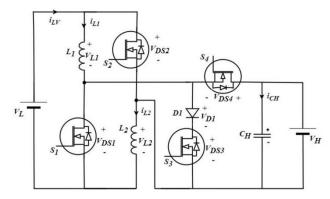
FIGURE 1. Proposed high gain bidirectional DC -DC converter (HGBDC).
