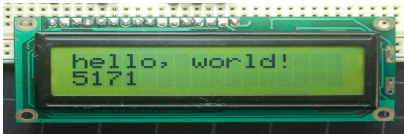
Output of the sketch on a 16x2 LCD
