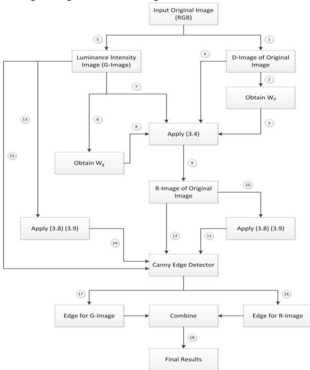
**Fig. 5.** Flowchart for Colour Edge Detection
